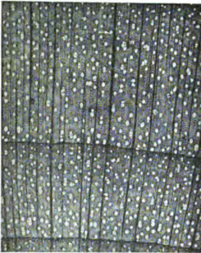
FIG. 1.—Cross-section of Diffuse-Porous Wood. (Hard Maple.) (Bull. 126, U. S. For. Ser.)
